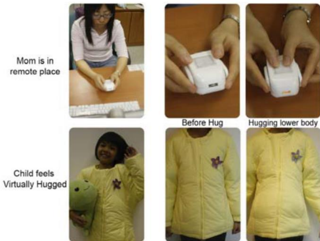
Figure 2.3 Huggy Pajama system overview. Reprinted from Huggy pajama: a parent and child hugging communication system (Teh et al., 2009). Copyright © Association for Computing Machinery.
