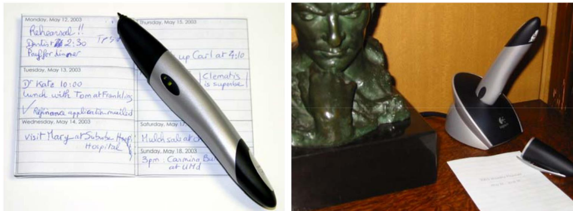
Figure 2.8 The prototypes of the digital paper and the pen. Reprinted from Shared family calendars: Promoting symmetry and accessibility (Plaisant et al., 2006). Copyright © Association for Computing Machinery.
